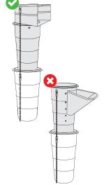
TOP HOPPER DO NOT start the column with a side hopper piece. Unsecured, loose or unscrewed hopper section
